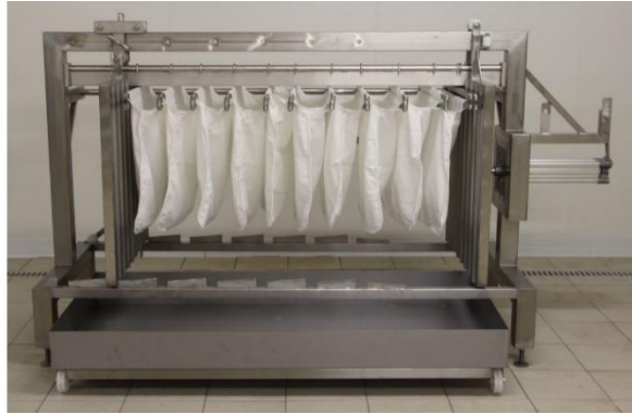
Figura 15 Press filter for lactic cheese, tomado de [76]
