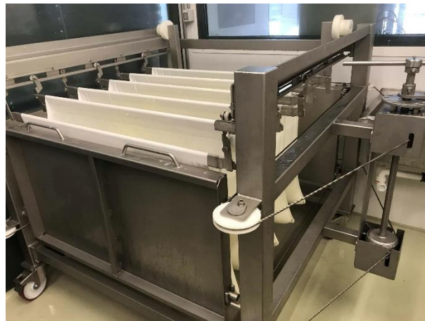
Figura 16 Filter press, tomado de [77]
